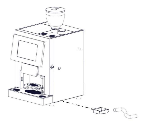
Then make a hole (diameter 7 mm) in the plastic drip tray (see image below). In this way the liquid collected, will be discharged externally through the tube that was previously connected (previous step).
