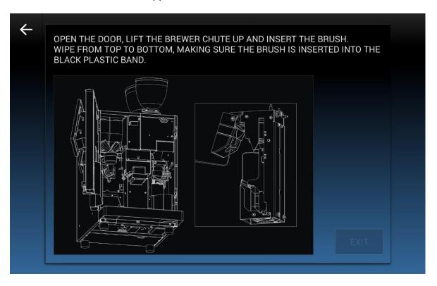
Once cleaning operations have been completed, the *Exit* key will be enabled. Insert Password 1111 in order to exit from the Cleaning Menu.
