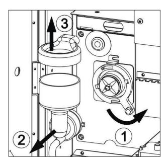
Rinse the parts under running water. Scrub thoroughly using the brush.
