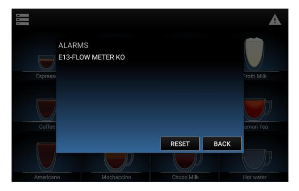
Push on the **FLOW METER KO** alarm and the following screen shot will appear. This happened because at the first initial water fill in of the machine, the water doesn't arrive directly to the boiler.
