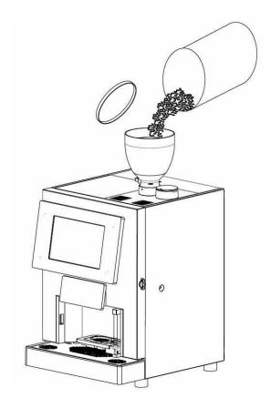
Remember to open the beans stopper located at the bottom of the coffee beans hopper. (see image A below).
