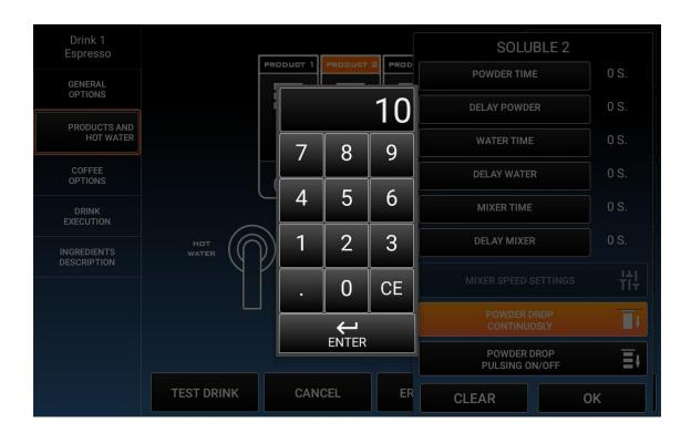
You can set the seconds for the mixer and after that, the key **Mixer Speed Settings** will be enabled.
