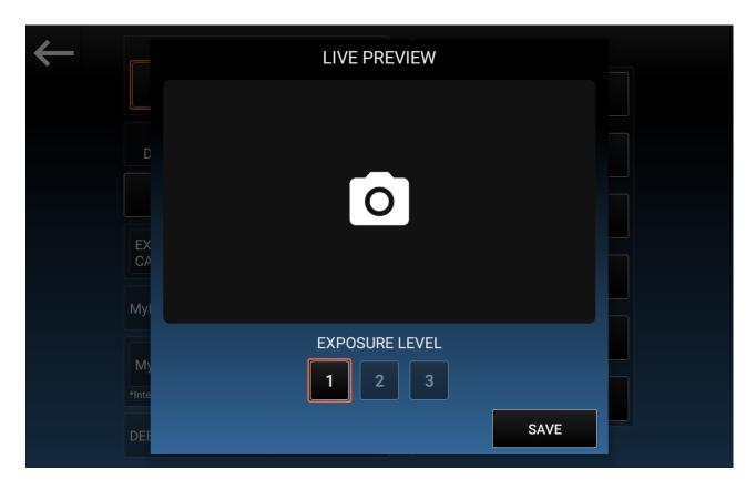
If the camera is connected properly, it will be shown a live preview. It is also possible to adjust the camera exposure to improve the code recognition performances, according on the ambient light;
