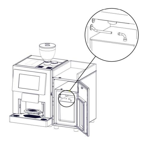
• Remove the milk container. Empty and rinse the container, the milk pipes and the filters.
