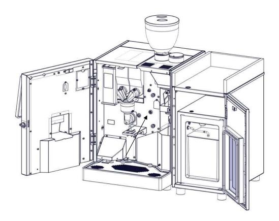
Connect the pipe to the black plug of the milk container as indicated on the image below
