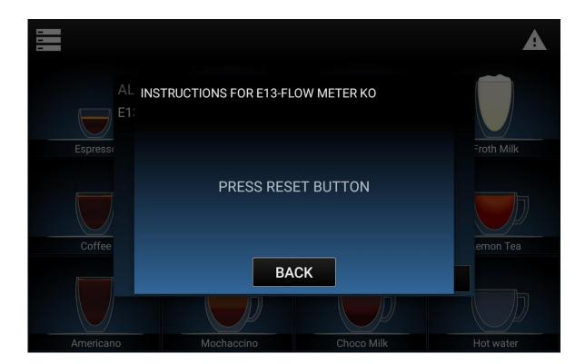
After the press of the RESET button the machine will load the boiler, and the Hydraulic Loading screen will be shown again.
