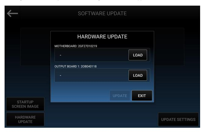
It is possible to **Load** the software for the boards from the touch screen memory or from an external USB drive.
