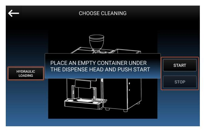
Push on the **Start** button to start the Hydraulic Loading procedure. This operation will take about 5 minutes.
