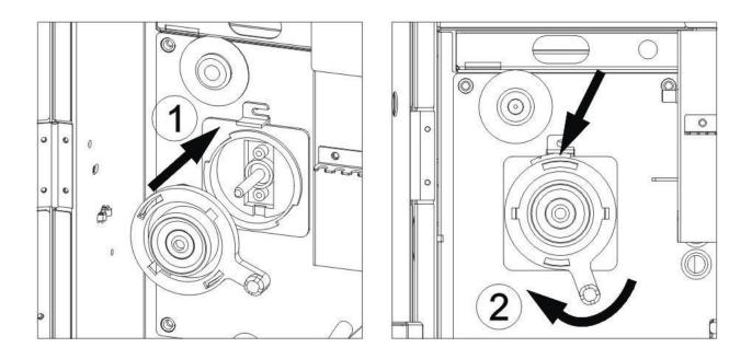
2. mixing blade Turn the shaft with the flat side up (1) and insert the mixing blade so that its internal flat side aligns with the one of the shaft.
