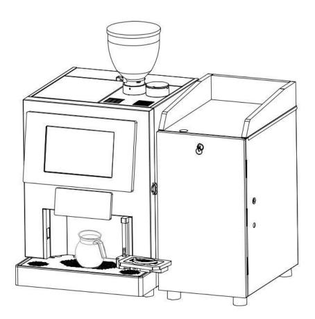
• Push **Start** when ready, the cleaning liquid will be discharged directly in the jug. The cleaning cycle will take about 15 minutes.
